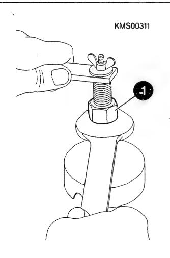
COMPONENT CHECKING AND REPAIR Checking commutator end shield Installation: Press new bushing with pressing-in mandrel (1) and locating sleeve (2) into commutator end shield from inside. Make sure locating sleeve (2) is properly positioned in commutator end shield. ATTENTION: Moisten new bushing beforehand with suitable oil. comm. avail. Mandrel press: Pressing-in mandrel: 0 986 617 149 Locating collar: 0 986 617 212
